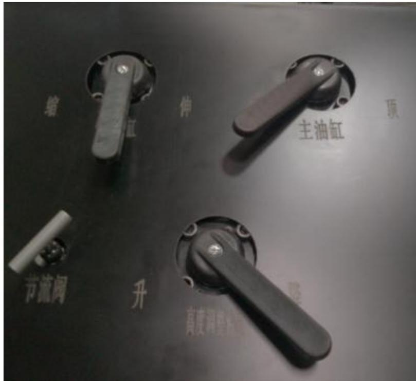
TIP: Strictly observe the "WARNING" statement in this instruction manual during retraction of the master cylinder. When operating the main oil retraction, the throttle valve V82 (1) must be fully closed
