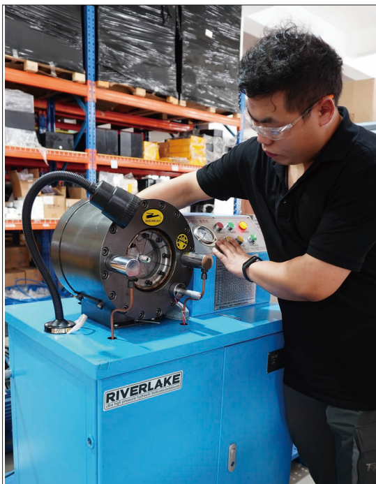
Hydraulic hose manufacturing
